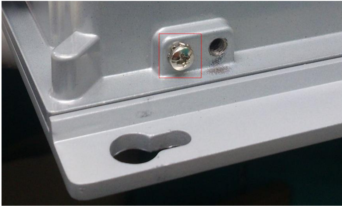
Ground screw of IES-5208DF switch
