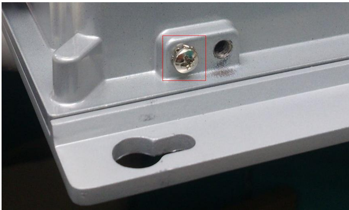
Ground screw of IPES-0008A switch
