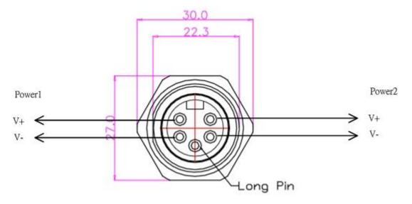
Pin assignment of Power input
