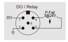
Pin assignment of alarm relay
