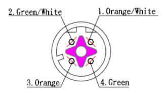
Pin assignment of M12 10/100Tx network connector
