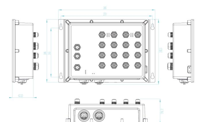
Aluminum case. IP-54, 285 (W) x 201.4 (D) x 84.4 (H) mm
