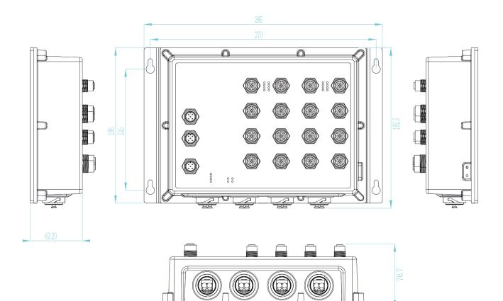
Aluminum case. IP-54, 252 (W) x 179.5 (D) x 91 (H) mm
