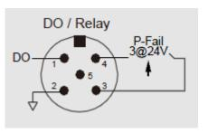
Pin assignment of alarm relay
