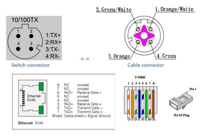
Pin assignment of M12 10/100Tx network connector
