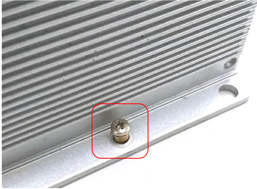
Ground screw of router
