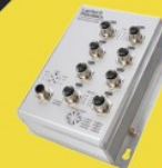
T(P)GS-0008CA 8 10/100/1000T (PoE at) EN50155 Unmanaged Switch
