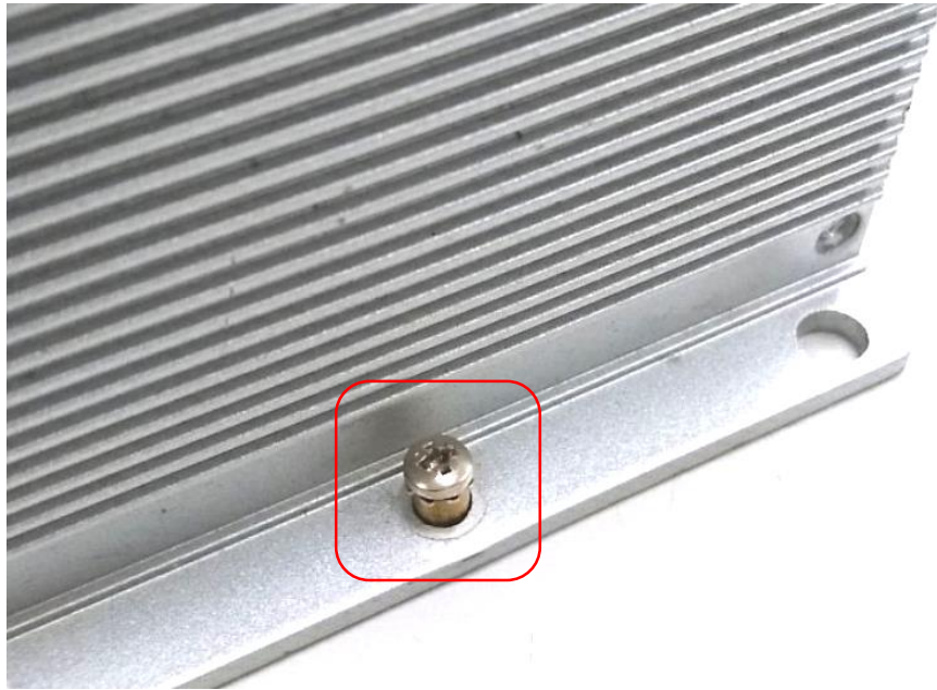
Ground screw of router
